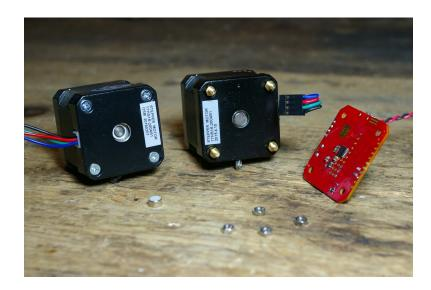
You will need to mount the magnet to the back of the motor shaft. *Note: the magnet must be diametrically magnetized, as opposed to axially magnetized.* The magnet may naturally stick to the shaft, but we recommend a dab of epoxy or super glue to hold it in place. The magnet should be fairly centered, but the calibration routine will correct for minor misalignment.
